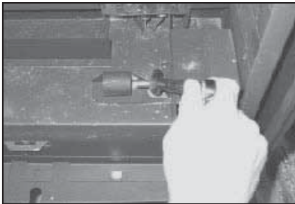
Figure 6.5 Remove main burner orifice using a 5/8 in. wrench. Replace orifice with the proper size as indicated on for your gas type and venting.
