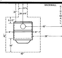
CHIMNEY AND ACCESSORIES: (Used through walls, ceiling and outside) dwelling). Use 7" diameter U.L. Listed factory built, residential type and building heating appliance chimney. Do not use Type B chimney which is used for venting gas appliances.
