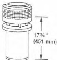
Termination Manufactured Home TF8-MHT
