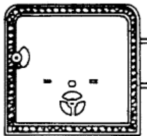
Fig. G-3 Side Door 46" (Extra Large), 40" (Small & Large) - \frac{7}{16} " fiberglass Seals side door to left side.
