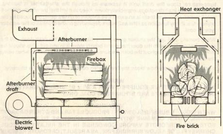
observe the fire's progress through the window above the firebox door. WARNING: Do not position your face closer than 12" from the window when the stove is in operation. When the kindling and small pieces of wood have formed a live bed of coals 4" to 6" deep, which may take as long as a full day of burning depending on the type of wood used, insert larger pieces of wood or coal being careful to keep a 2" clear area all around the afterburner.
