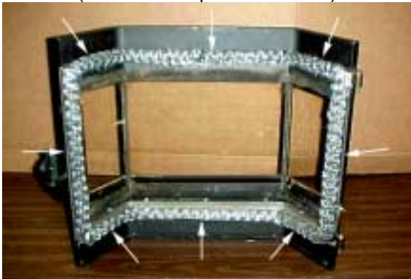
Door Rope Gasket (check seal at points indicated)
