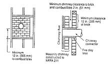
A Minimum 3.5-in thick brick masonry all framed into combustible wall with a minimum of 12-in brick separation from clay liner to combustibles. The fireclay liner shall run from outer surface of brick wall to, but not beyond, the inner surface of chimney flue liner and shall be firmly cemented in place.
