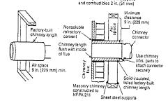
Minimum chimney clearance from masonry to sheet steel supports
