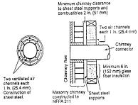
C Sheet steel chimney connector, minimum 24 gauge in thickness, with a ventilated thimble, minimum 24 gauge in thickness, having two 1-in. air channels, separated from combustibles by a minimum of 6-in. of glass fiber insulation. Opening shall be covered, and thimble supported with a sheet steel support, minimum 24 gauge in thickness.
