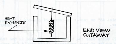
Note: Mark inlet and outlet on top of tank (see heat exchanger illustration).
