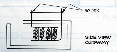
Now lower the Heat Exchanger until the crosspiece supports it. The Heat Exchanger should NOT be resting on the tank bottom.
