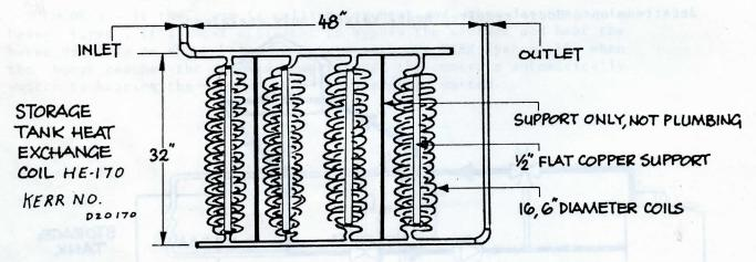
Coil rating should be 170,000 BTU/h at 40 F temperature differential and 10 gallons per minute(U.S.). A typical coil with 1 1/4" connections, as illustrated above would consist of 4 coils of 1/2" finned copper 16 turns in 32 inches. NOTE — This type of coil is recommended to ensure good heat transfer when taking heat from storage.
