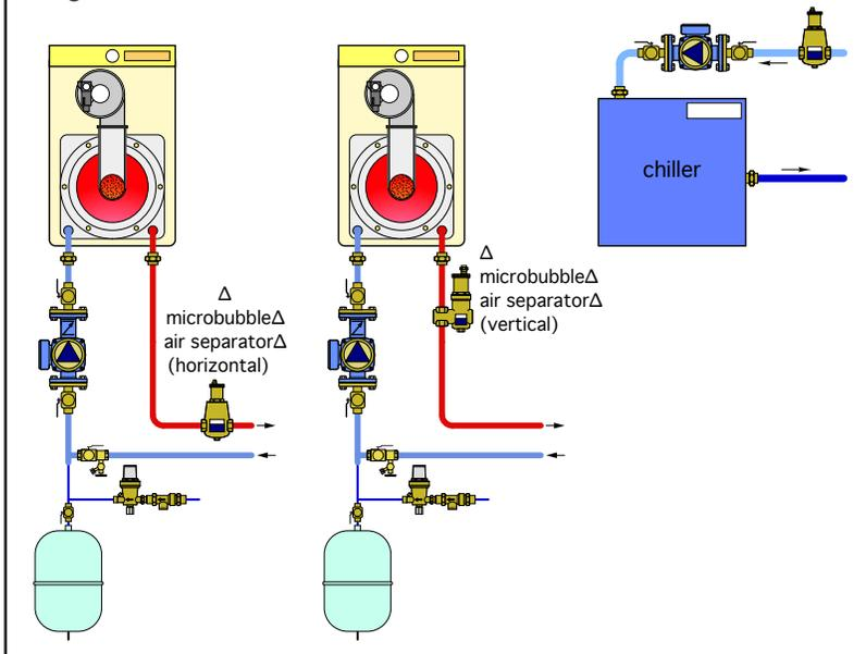
As microbubbles coalesce together, they form larger bubbles. Eventually, the bubbles attain a volume large enough that buoyancy forces overcome the adhesion forces holding them to the coalescing surface. The bubbles then rise along the coalescing surfaces to a chamber above the main flow stream where they can be collected and expelled through a float-type air vent. The concept of coalescence inside such a separator is illustrated in Figure 2-22b.
