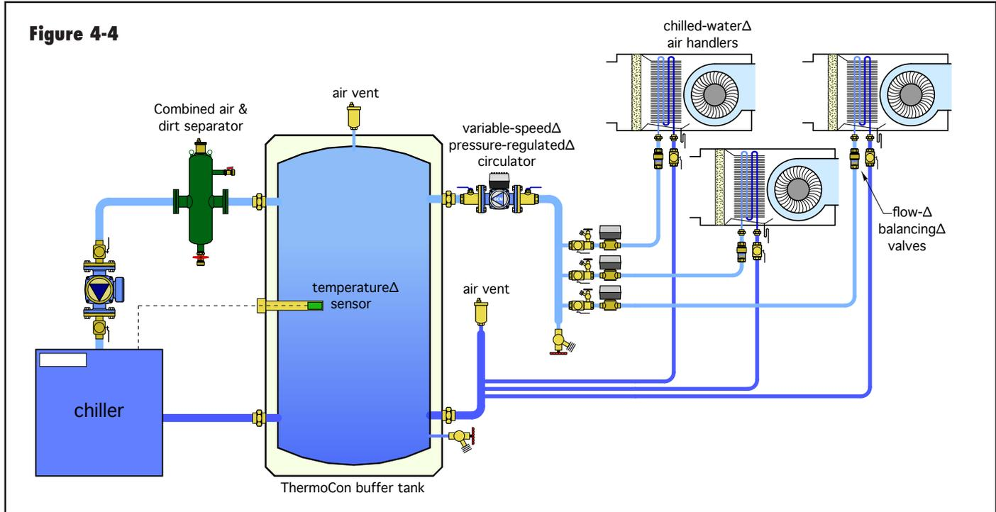
**PLACEMENT OF COMBINED AIR & DIRT SEPARATORS**
