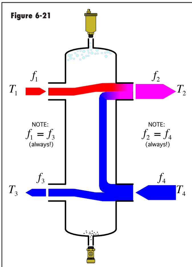
same time, the boiler flow rate is 10 gallons per minute, and the water temperature supplied to port 1 is 160°F. Determine the mixed water temperature leaving port 3. Also, what is the water temperature returning to the boiler?
