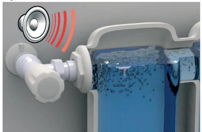
Entrapped air sounds often become noticeable as flow begins to disturb stationary air pockets. Air-filled cavities within piping and radiators act as acoustic amplifying chambers, especially if water enters a component which has trapped a large pocket of air. Noise is also generated when dissolved gases within water are released due to a sudden drop in pressure. This is called gaseous cavitation, and it often occurs at the orifice of valves or the inlet of circulators.
