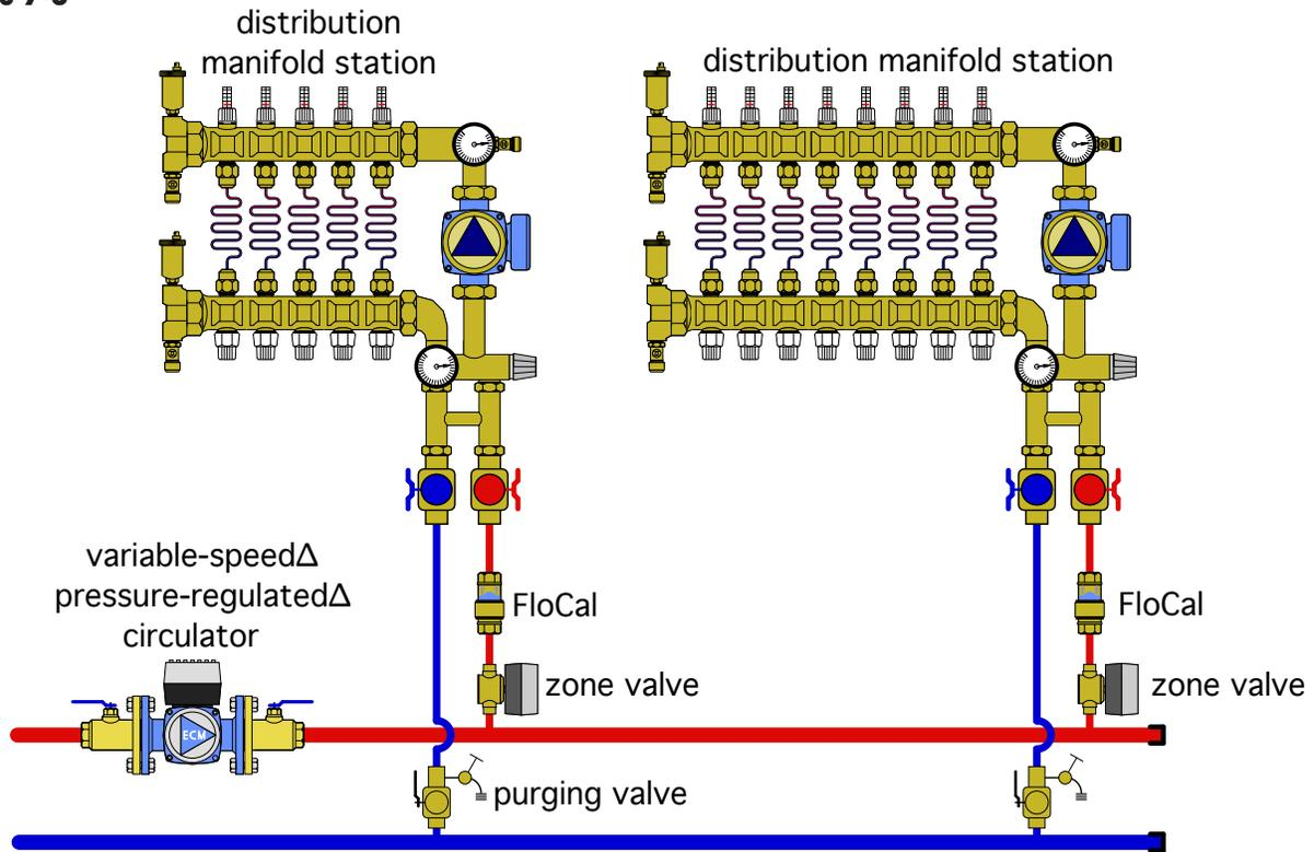
station. The “crossover” tubes just above the isolation ball valves on each manifold station allow hydraulic separation between the built-in manifold station circulator and the variable-speed pressure-regulated circulator that supplies flow in the headers. This arrangement also allows the option of continuous flow through the distribution circuits connected to the manifold stations. The mixing
