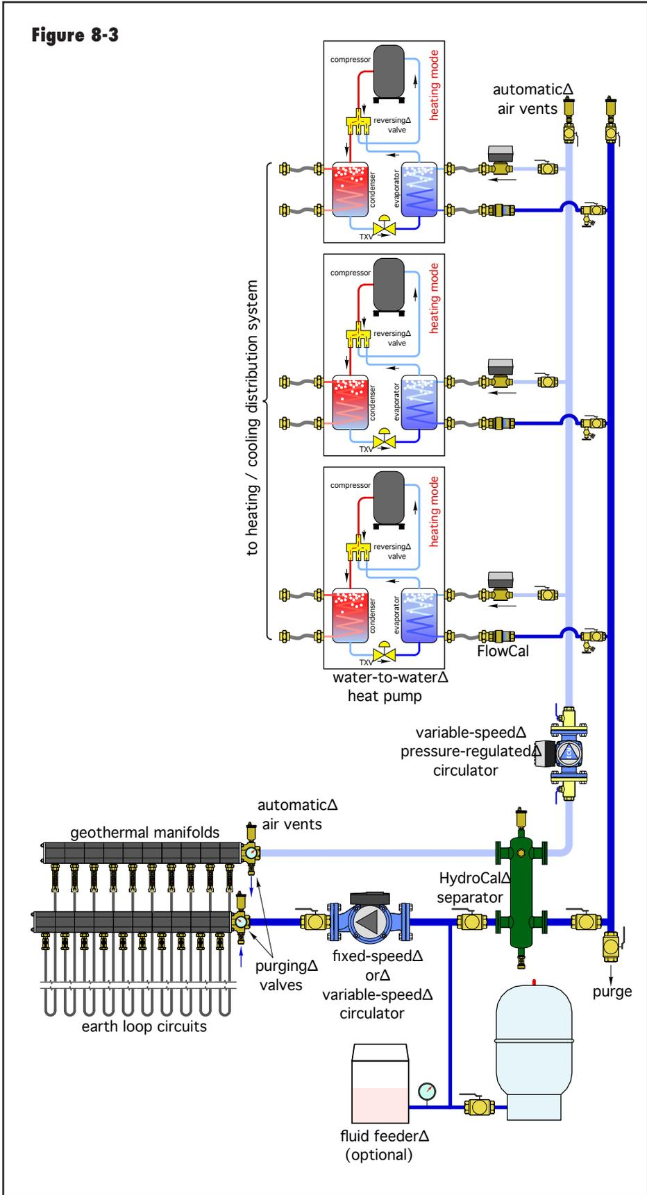
closing of zone valves or motorized ball valves on each heat pump. The earth loop circulator could also vary its speed in response to some control criteria, such as the temperature drop or rise across the earth loop connections to the hydraulic separator. This allows the power required by the earth loop circulator to be reduced as the number of operating heat pumps decreases.
