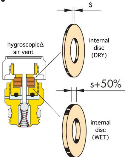
When the knob is fully closed, an internal O-ring seals off the side port. However, if air is present at the vent, the fiber discs will dry and allow air to pass through them. This air is discharged under the vent’s knob, as shown in Figure 2-19b. Once the air has been vented and water reaches the fiber discs, they swell very quickly to seal off any further discharge.
