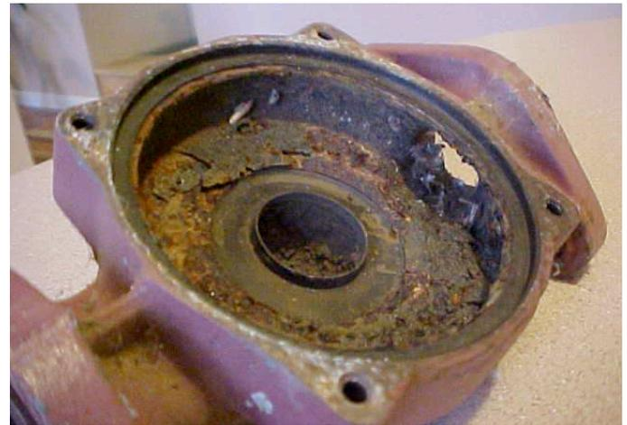
If oxygen continues to be present in the system, magnetite will be converted to hematite (Fe<sub>2</sub>O<sub>3</sub>), which can cause pitting corrosion throughout the system.
