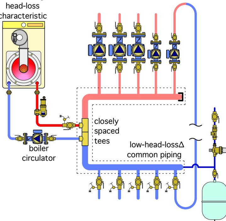
One solution is to couple such heat sources to a generously sized header system using a pair of closely spaced tees, as shown in Figure 6-4.
