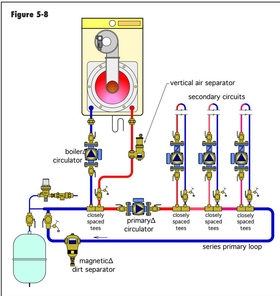
whenever two or more of the secondary circuits are operating simultaneously. Although there are situations in which this temperature drop doesn't present a problem, it does add complications that designers must assess and compensate for.
