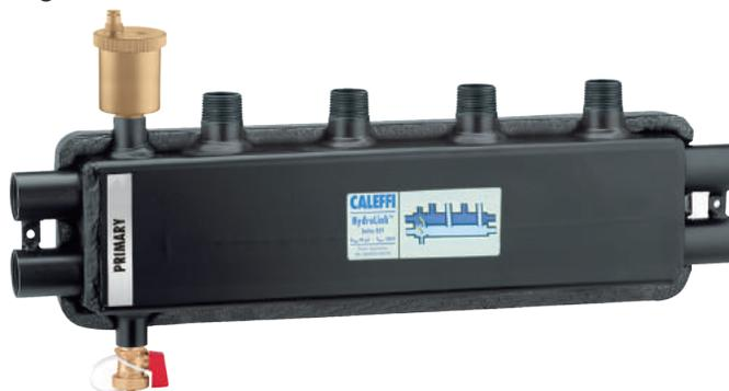
The HydroLink provides a chamber to hydraulically separate the boiler circuit from the distribution circuits. It also provides a self-contained manifold station that supplies up to four independently controlled load circuits with the same supply temperature. These features and their equivalent piping are shown in Figure 7-2.
