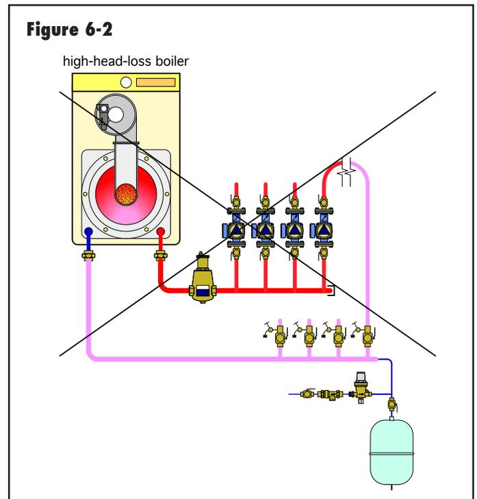
The high head loss of the mod/con boiler significantly increased the overall head loss of the common piping and largely negated the hydraulic separating characteristic attained in systems using the older style, low-head-loss boilers. This created many problem installations, since installers and manufacturers did not immediately recognize the source of the resulting flow problems.
