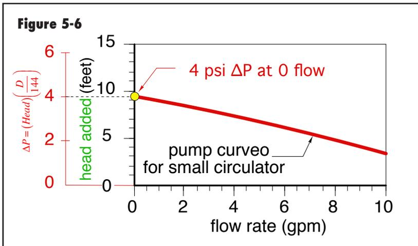
Figure 5-6 shows the pump curve for the smaller circulator. Notice that the maximum possible differential pressure this circulator can create is 4 psi.
