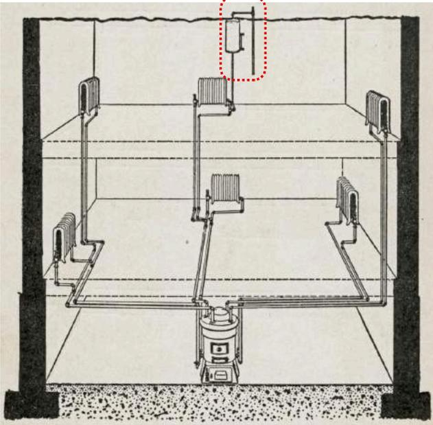
system—usually in the attic or upper floor, as seen in Figure 2-1, which appeared in a heating design manual published in 1906.
