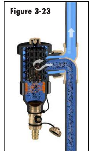
Figures 3-22 and 3-23 shows another variation on a magnetic dirt separator. In this case, the separator's body is made of engineered polymer. The body connects to a rotatable brass base fixture that allows the body to remain vertical regardless of the orientation of the pipe to which it is attached. This separator also contains a media that helps separate dirt from the flow stream. The magnetic collar can be seen at the lower end of the body.
