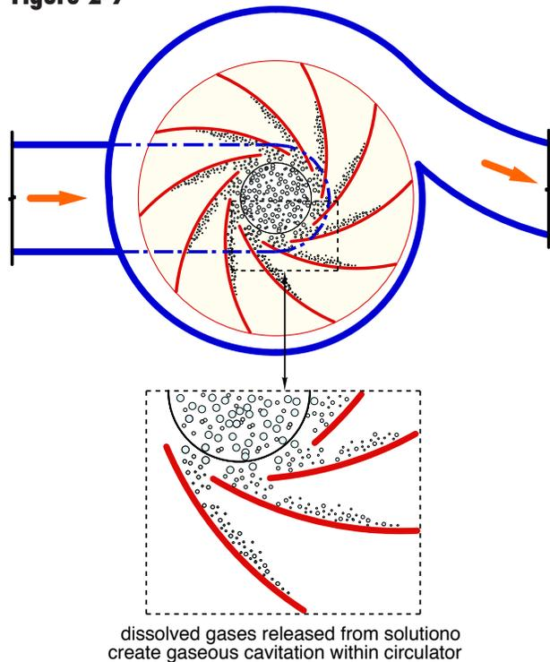
of air. If a sufficient volume of air enters the volute and displaces water in the impeller, the circulator may be unable to clear itself and will quickly be running without lubrication. Failure is almost certain.
