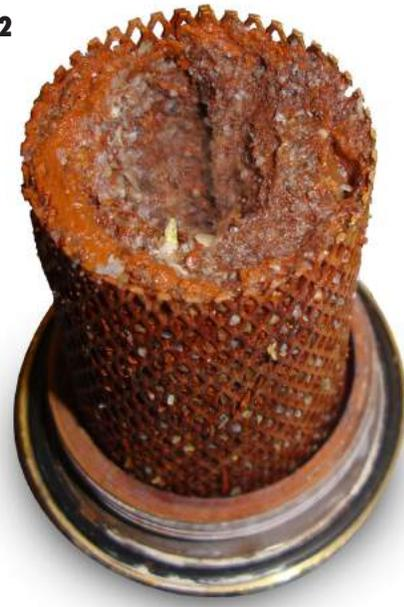
Flow reductions due to dirt accumulation in Y-strainers will reduce heat conveyance by the system. When restricted strainers are present near the inlet of circulators, they can induce vapor cavitation due to significant pressure drop. This can severely damage a circulator if not corrected.
