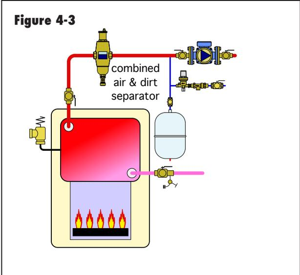
Combined air & dirt separators use the same principles of microbubble air separation in the upper portion of the separator body, combined with low-velocity-zone dirt separation in the lower portion of the separator body. They have a float-type automatic air vent at the top of the body and a drainage valve at the bottom, as seen in Figure 4-1.
