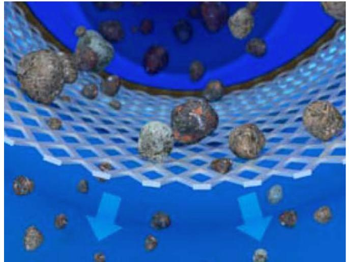
As debris collects inside the strainer’s basket, it impedes flow. This results in increased pressure drop and hence higher head loss. If the strainer basket is not properly maintained, such head loss can be excessive. Figure 3-12 shows an example of a heavily loaded basket from a Y-strainer.
