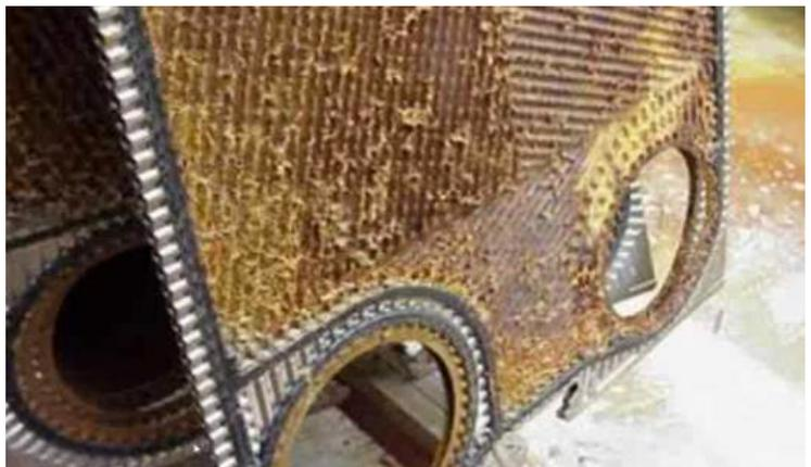
Similar fouling can occur with chillers and heat exchangers in chilled-water cooling systems.
