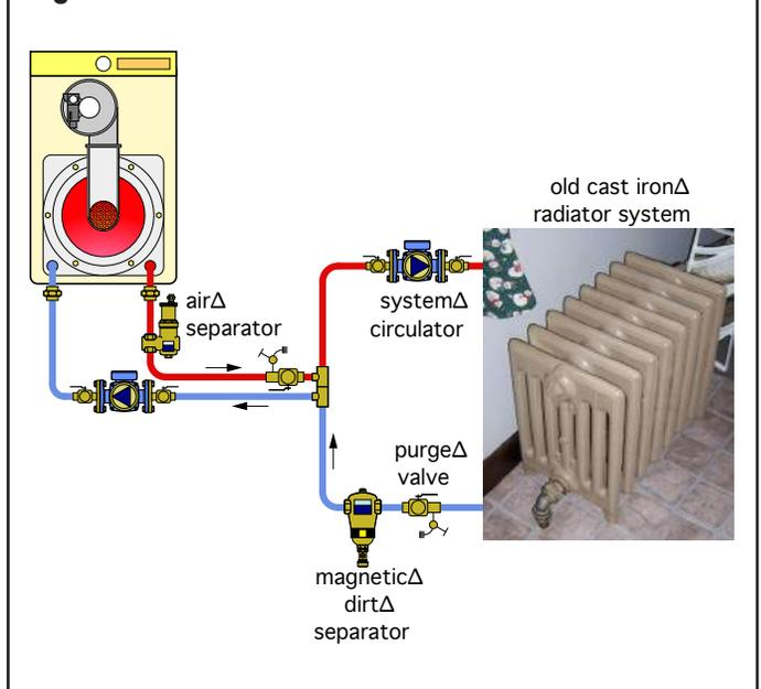
as shown in Figure 3-26. This is especially important in systems using boilers or other heat sources with compact heat exchangers. It's also very important in systems where a new boiler is installed in a system containing older piping and/or cast iron radiators, as shown in Figure 3-27.
