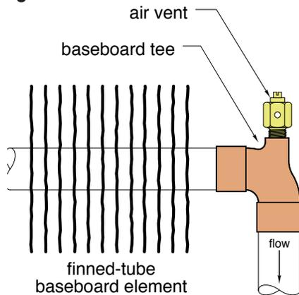
fittings resemble a 90° elbow, but with an extra port having either 1/8” or 1/4” FPT threads. They are typically installed at high points where piping changes from vertical to horizontal. Their name comes from a common application in which they are mounted on the outlet of a fin-tube element within a baseboard convactor, as seen in Figure 2-16b.
