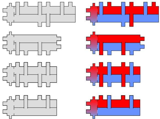
A typical configuration for the Hydrolink has the heat source connected to the “primary” chamber piping on the left side of the unit, along with several load circuits connected to the other “secondary” connections that connect into the manifold chamber. Two additional tapped connections are provided in the top and bottom
