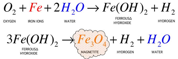
The compound Fe<sub>3</sub>O<sub>4</sub> is called magnetite and appears as a dark gray sludge within the system. Magnetite is also attracted to magnetic fields created by circulators, especially those containing powerful permanent magnets. Circulator manufacturers have developed improved methods of forestalling magnetite or other ferrous metal particles from reaching the rotating inner parts of their circulators, but the potential for some magnetite entry into such parts still exists.
