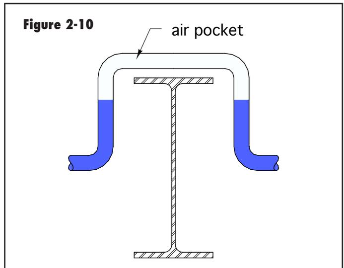
can form at the top of heat emitters, boiler sections, unvented tanks, inverted diaphragm-type expansion tanks or heat exchangers. Air pockets can also form in horizontal piping that eventually turns downward or piping that is routed above obstacles in its path, as shown in Figure 2-10.
