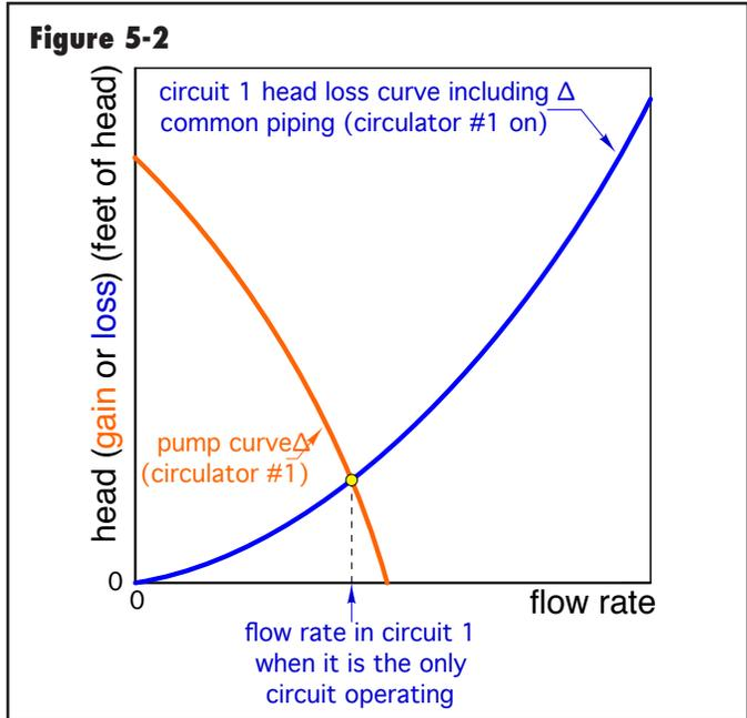
Next, assume circulator 2 is turned on, while circulator 1 remains on. The flow rate through the common piping increases, and so does the head loss across it. However, because of its spacious geometry, the increase in head loss across the common piping is very small. The system head loss curve that is now "seen" by circulator 1 will steepen, but very slightly. It is shown as the green curve in Figure 5-3.
