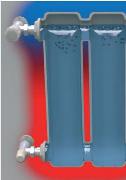
**Accelerated Corrosion:** Air is about 23% oxygen, and oxygen in contact with ferrous metals such as steel and cast iron causes corrosion. Many improperly deaerated
