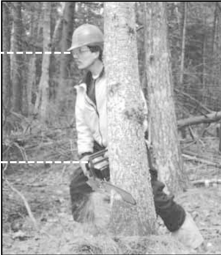
The sight line on the saw can be used like a gun sight to determine an exact falling direction for the tree.
