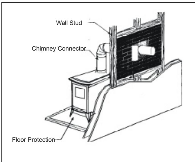
Fig. C: An example of an approved wall pass-through
