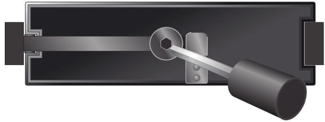
To remove the ashes from the stove, push them down through the centre grate using the tool provided. Place ashes in a metal container with a tight fitting lid. The closed container of ashes should be placed on a non-combustible floor or on the ground, well away from
