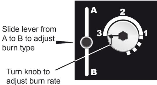
Use the tool provided to adjust the stove's air controls
