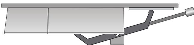
Post-combustion and airwash shutters open, providing top air for optimal wood burning. Under-grate air flap closed.
