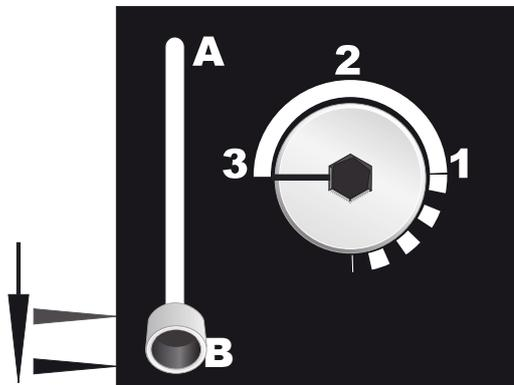
The burn rate knob is rotated fully counter-clockwise to supply the stove with the maximum quantity of air because the flue will be cold. The burn type lever is set to its lower position to supply air to the fire from beneath the grate, accelerating the speed at which the fire size increases, as well as air above the fire to burn the volatile matter, reducing the smoke and lessening the production of glass staining tars.
