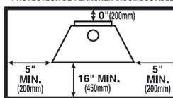
FLOOR PROTECTOR MUST BE A NON-COMBUSTIBLE MATERIAL, AND IT MUST EXTEND BENEATH HEATER, AND TO THE FRONT/SIDES/REAR AS INDICATED.
