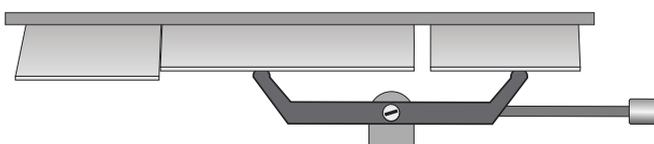
All air shutters open, providing maximum air intake above and below grate for ignition.
