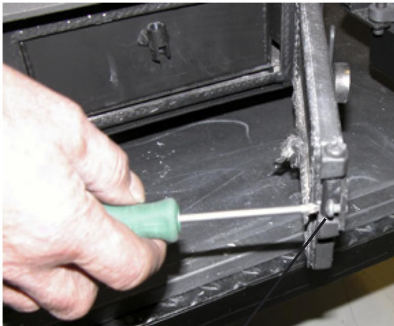
Adjust the screw at the end of the ash pan door lever to give a positive action when closing. Do not over adjust. The closing action of the lever should have a gentle resistance.
