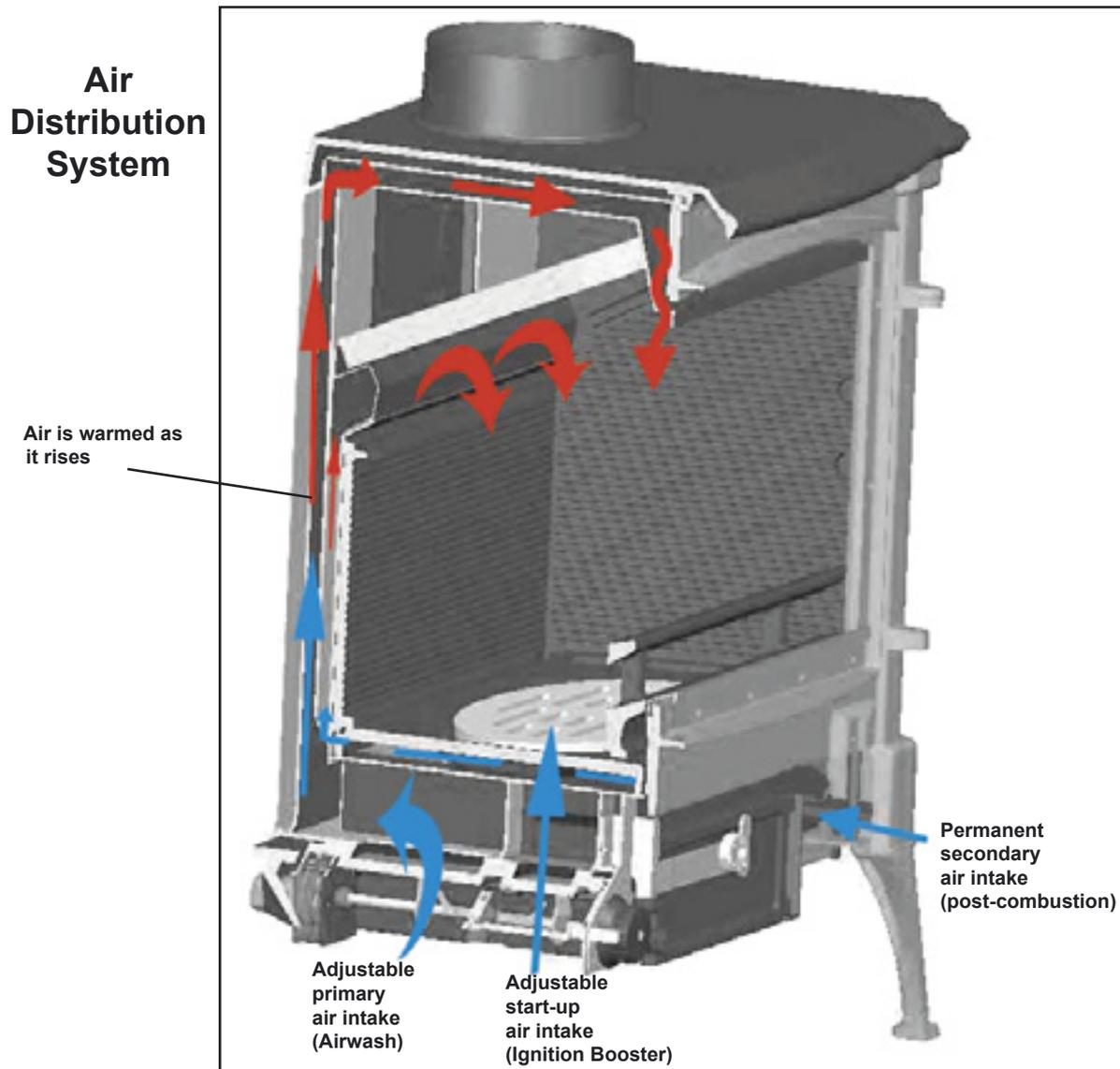
Note: For the purpose of clarity, the refractory bricks lining the firebox are not shown in the illustration above.
