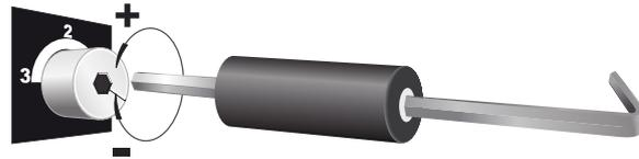
As the knob is rotated counterclockwise, the cam progressively opens the air shutter to allow an increasing amount of air into the stove.
