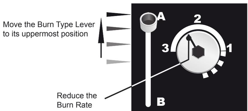
As the fire grows and the flue warms, the Burn Type Lever can be moved in one or two stages to its uppermost position (A), and the Burn Rate Knob moved progressively (clockwise) to lower settings. Much will depend on the quality of the wood being used and the performance of the flue but the stove will normally be operating with the Burn Type Lever at position "A" and the Burn Rate Control reduced within a few minutes of lighting.
