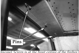
Inconel Screen is at the front ceiling of the firebox near the viewing window. Release the three pins to remove for a thorough cleaning.
