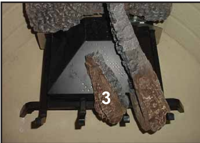
LOG #3 (SRV750-706): Place log #3 with the base on the inner right grate tine. The top of the log should be placed so that it doesn't cover any ports on the burner.
