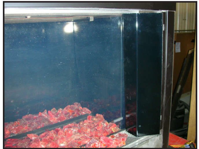
Figure 17. Outside Corner Trim Piece Installed.
