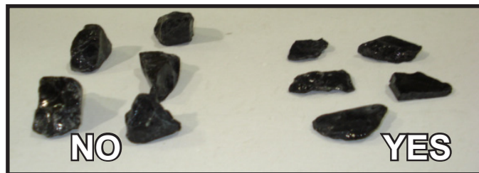
Figure 1. Selecting Flat Rocks for Pilot Cover
