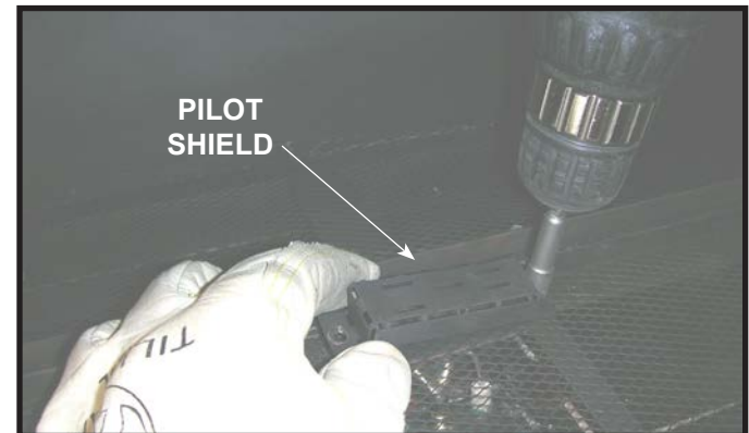
Figure 10. Removing Pilot Shield.
