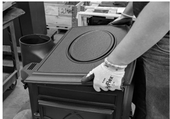
Fig. 21. Remove the top plate from stove.
