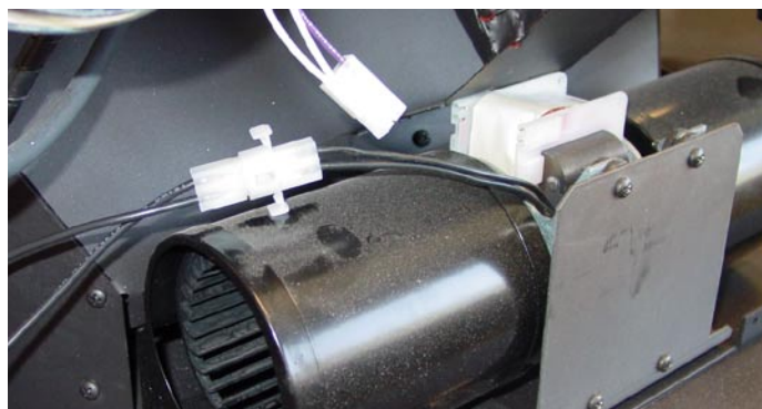
TEST CORD CONNECTED TO THE BLOWER
