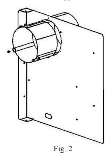
STEP 2: Attach the inner and outer telescoping vent pass through heat-shields to the wall plate as shown in Fig. 1 & 2. The vent pass through heat-shields are to be installed where the vent passes through the first adjacent wall to the left or right of the corner install kit.
