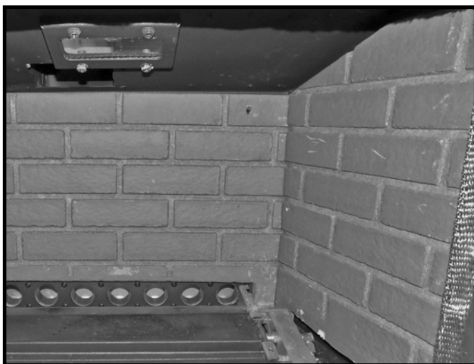
Figure 28: Right side panel in place.
