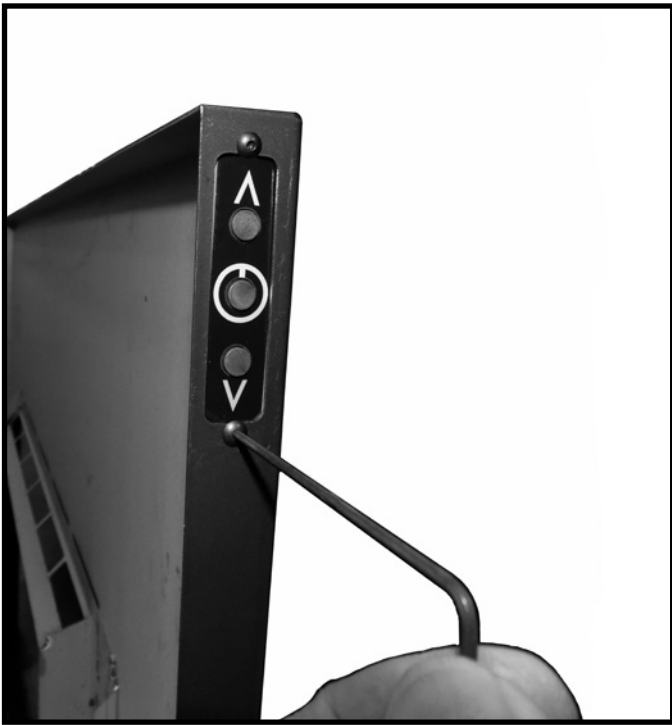
Figure 87: Attaching switch to backing plate.
