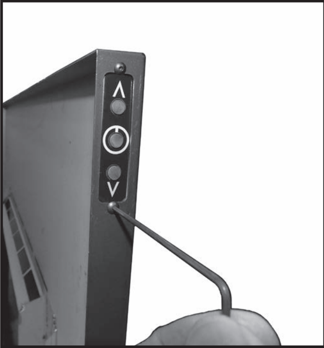
Figure 81: Attaching switch to backing plate.
