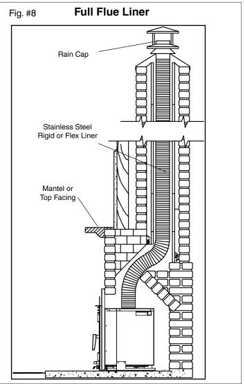
**Full Flue Liner:** where a listed stainless steel rigid or flexible liner extends from the Insert flue collar to the top of the chimney. **Direct Flue Connection:** where a listed stainless steel rigid or flexible liner extends from the Insert flue collar to the first chimney flue liner tile.
