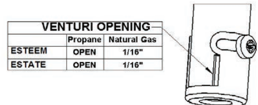
Figure 41: Venturi Shutter
