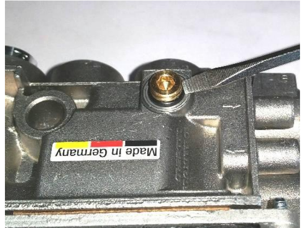
Figure 23 – Low Flow Orifice Removal – O-ring
