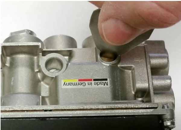
Figure 26 – Tighten LP Low Flow Orifice
