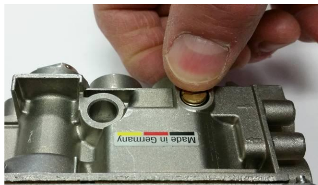
Figure 24 – NG Low Flow Screw Removal
