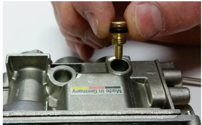
Figure 24 – NG Low Flow Screw Removal
