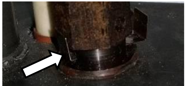
Figure 28 – Loosen Tower and Slide Pilot Gate to Rear of Pilot Tower (LP position)
