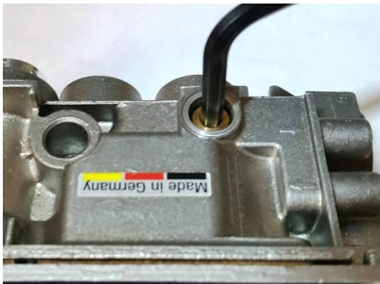
Figure 22 – Low Flow Orifice Removal
