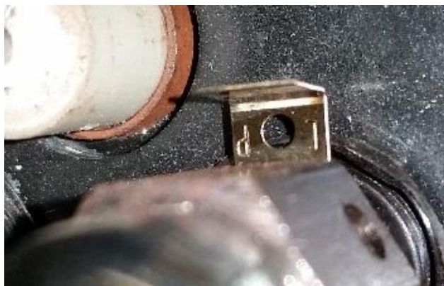
Figure 29 – Pilot in LP (LP text visible to rear of Pilot Tower)
