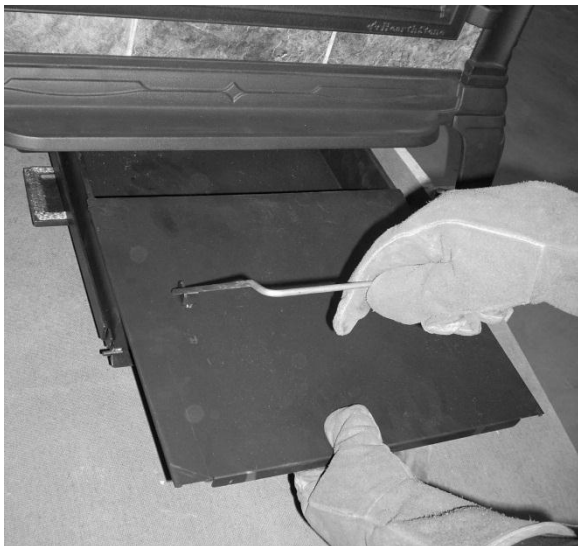
Image 1 – Slide lid onto ash pan
