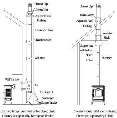
Figure 5 - Typical Venting Configurations
