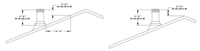
Figure 6 - Chimney Height Requirements
